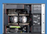
The ThinkStation P920 and P720 are built to support dual Intel Xeon scalable processors and up to the new NVIDIA Quadro RTX 8000 graphics inside.
