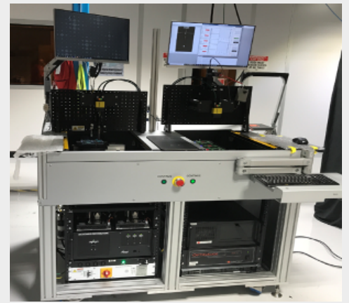
Automated, in-line stack metrology — Optical KPIs, Quality control
